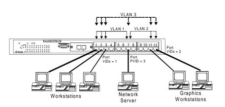
In the above example, there are three different VLANs and each port can transmit packets on one of them according to their Port VLAN ID (PVID) number. However, a port can receive packets on all VLANs (VID) that it belongs to. The assignments are as follows:
